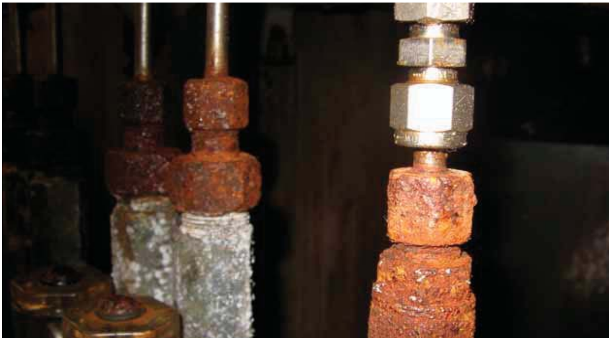
Galvanic reaction created by mixing different body & nut materials.
