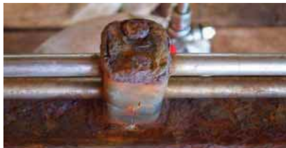
Crevice corrosion between the tube/tube trap interface.
