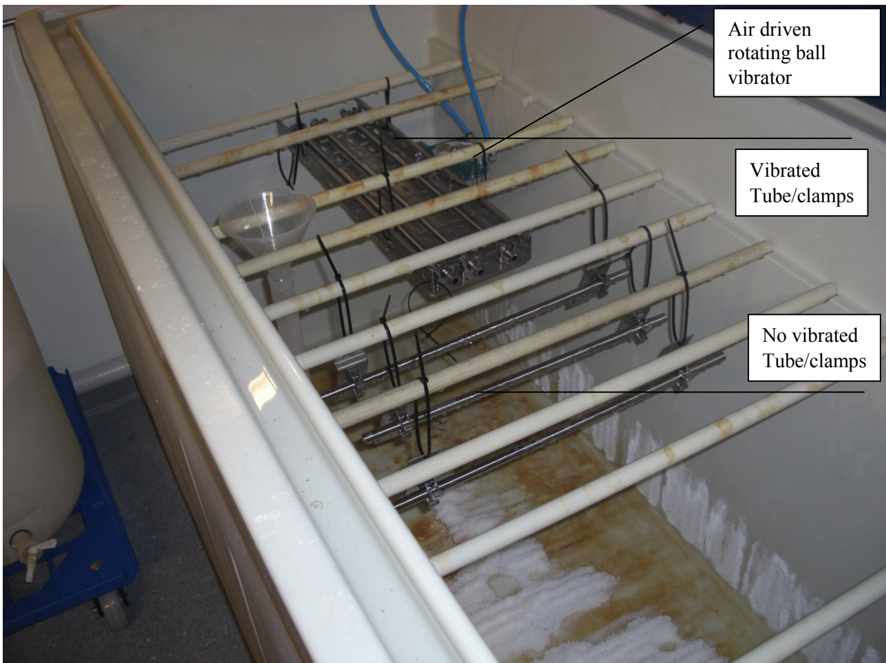
Figure 1 Picture of the test specimens inside the salt spray chamber.
